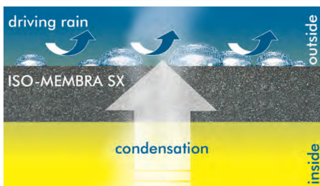
Performance principle of membrane seal
